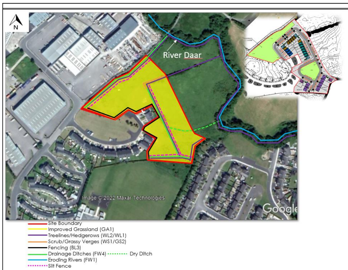
Figure 5 Habitat Map with proposed Silt Fence position to prevent run-off to drains containing water.
