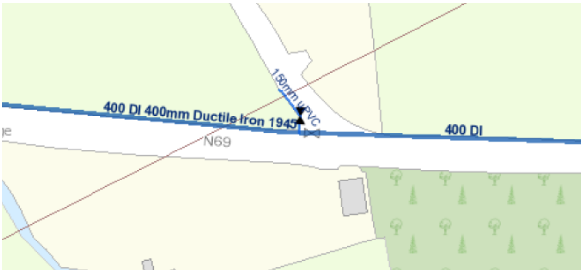
Figure 21: Irish Water pipes - plan
