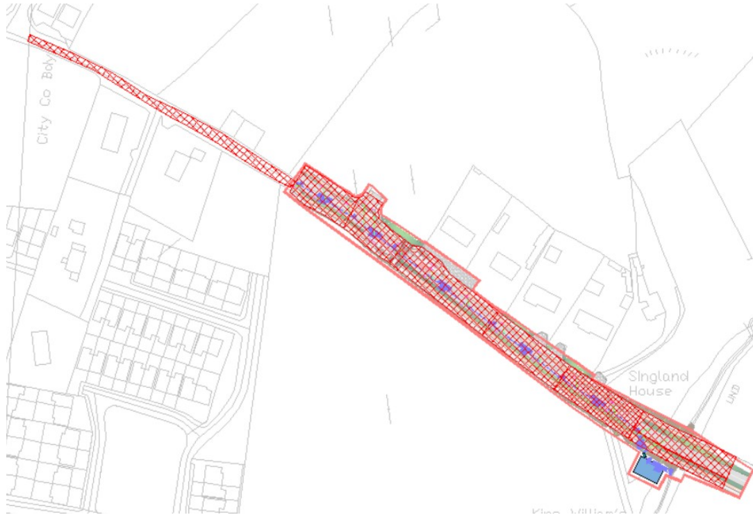
Figure 2: Proposed Drainage System Catchment Area
