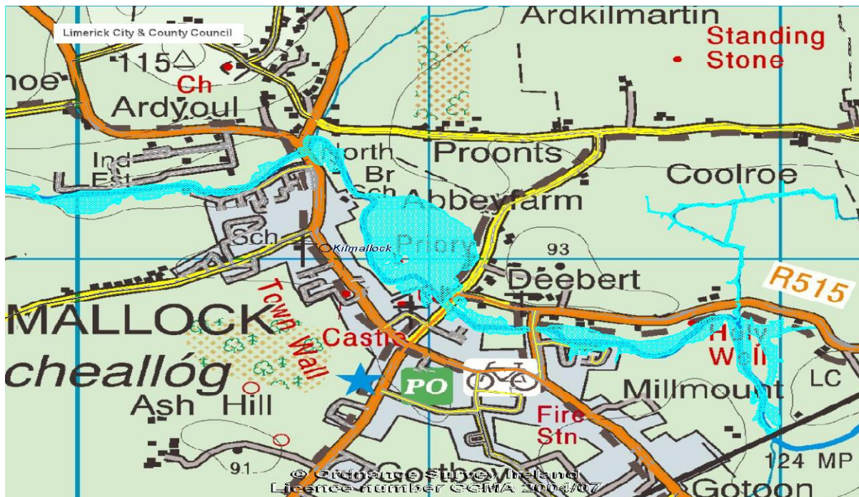
Figure 4: Screen grab of CFRAMS map showing areas at risk of flooding. These are along the Loobagh River and show the 1:100 flood risk areas.
