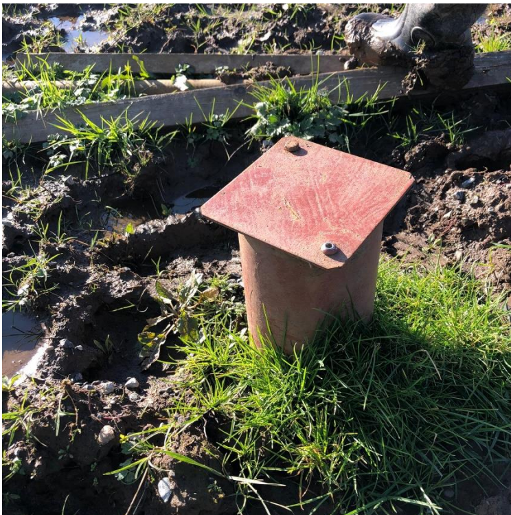
Image 7: Photograph taken of BH211. Wellhead is locked, protective fencing can be seen on the ground.
