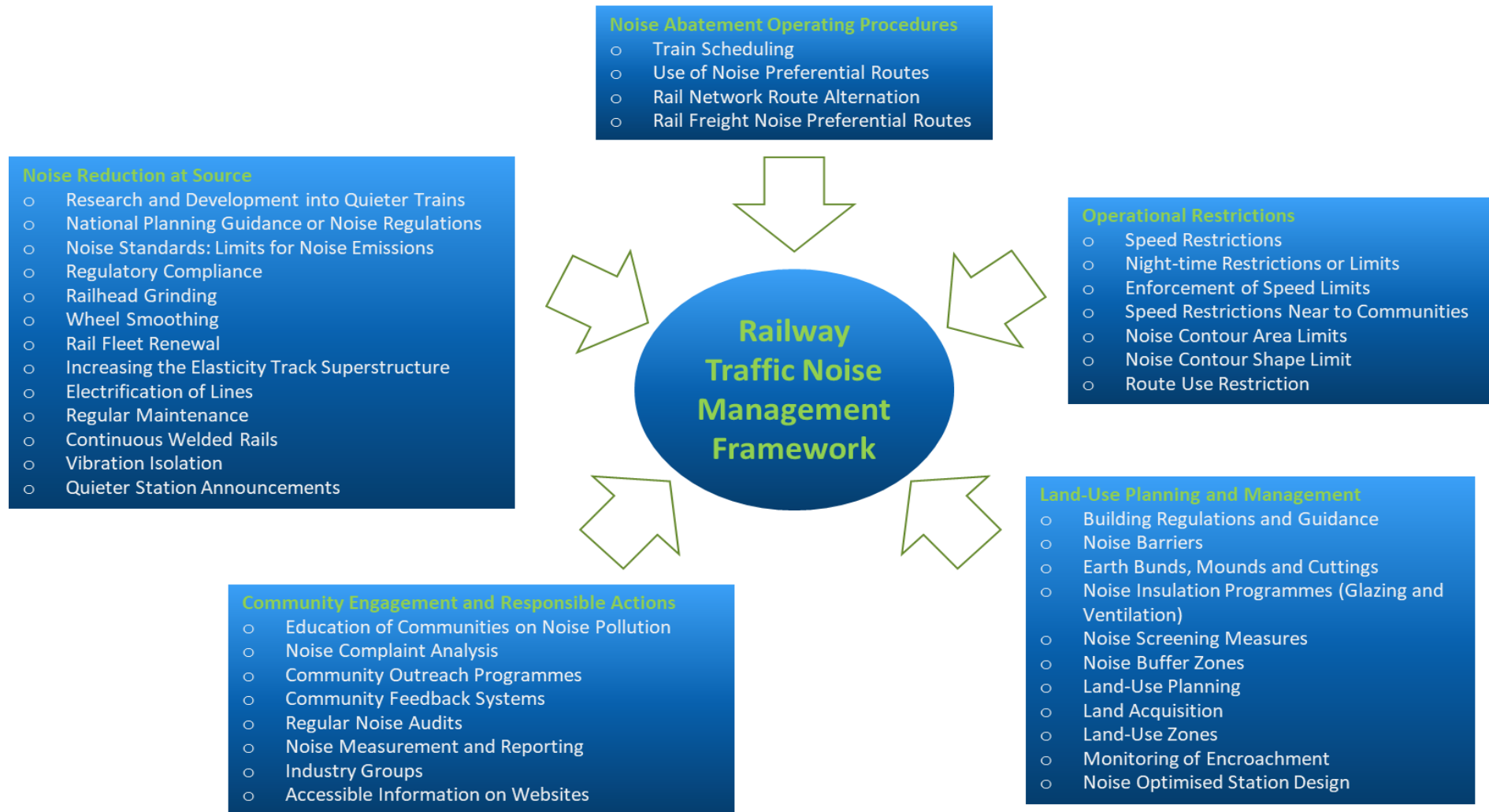
Figure 7.2. Railway Traffic Noise Management Framework.
