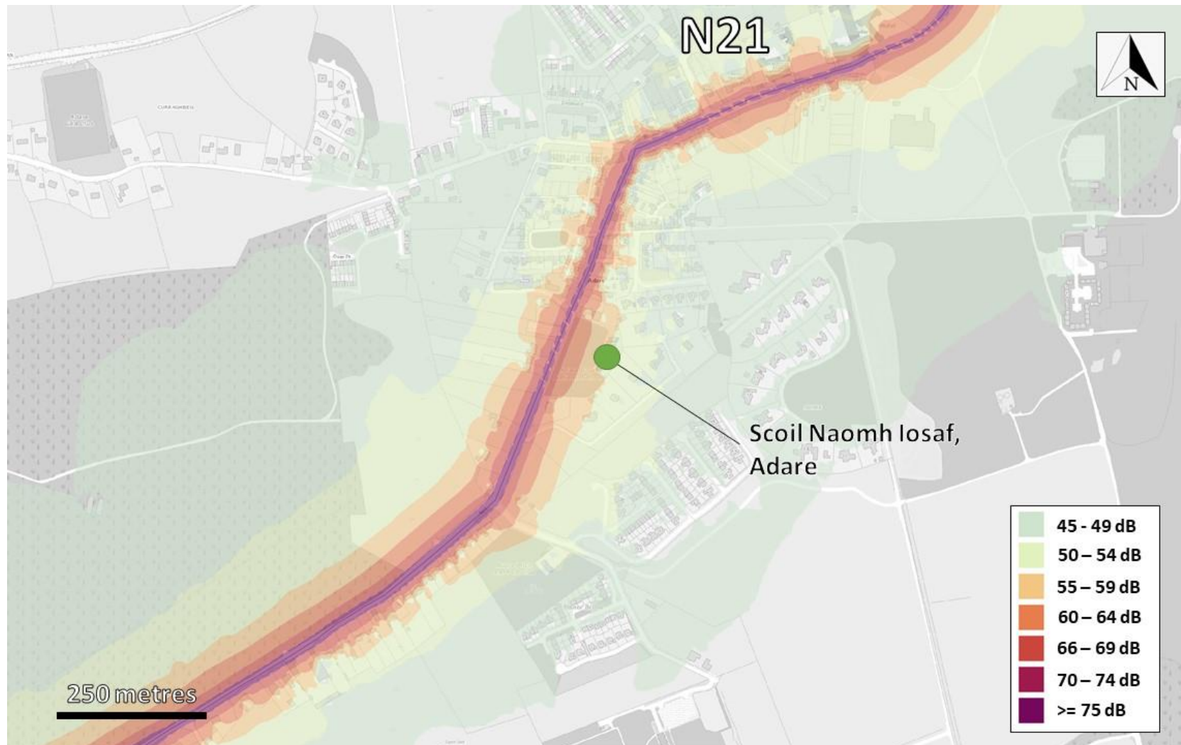
Figure D.6. L_{\text{night}} (dB) – N21, Noise Sensitive Buildings in the Adare Area.
