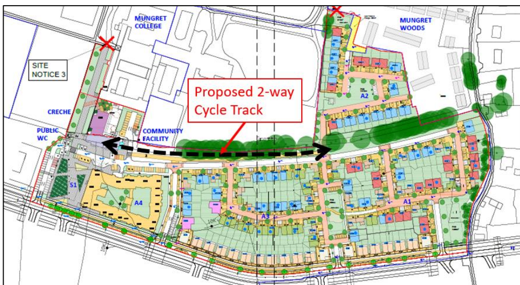
Figure 6 Proposed Two-Way Shared Pedestrian and Cycle Path
