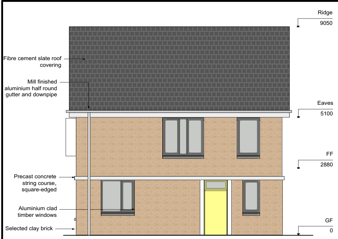
3B-5P Corner Brick Elevation A
