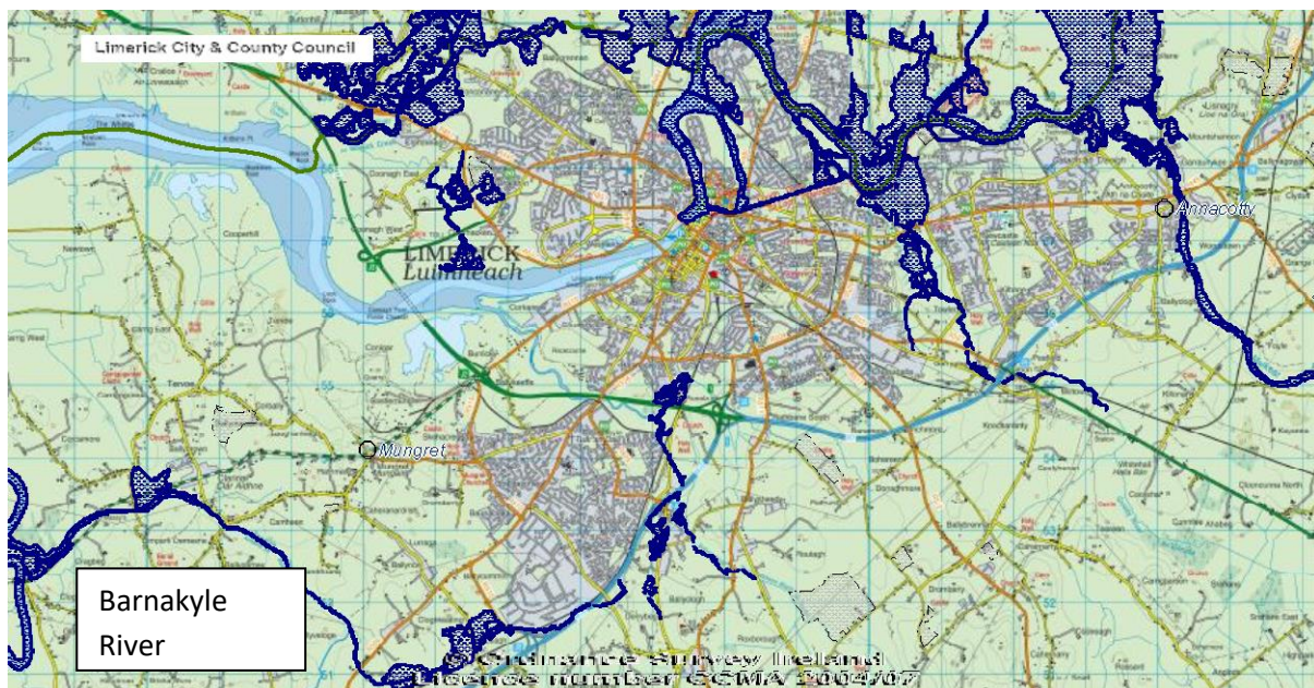
Figure 1: Taken from the LCCC planmap, this shows the extent of CFRAMs fluvial risk in the Southern Environs
