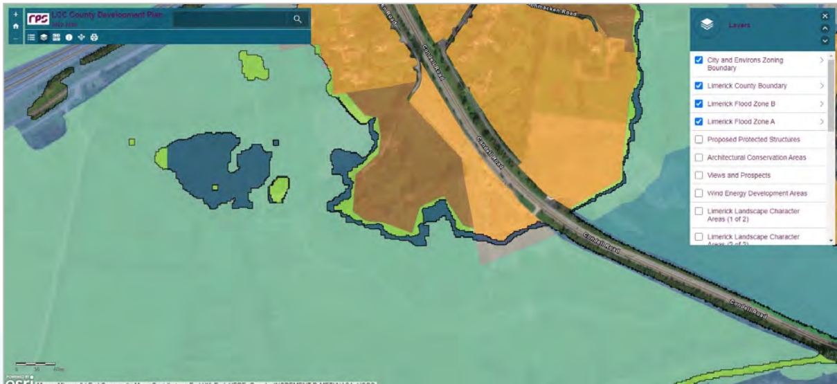
Figure 3: Proposed New Residential Zoning (brown colour), Existing Residential Development (orange colour) and Flood Zones A (light blue colour) and B (dark blue colour) overlaid on map. Source: LCCC Virtual Room - Interactive Map
