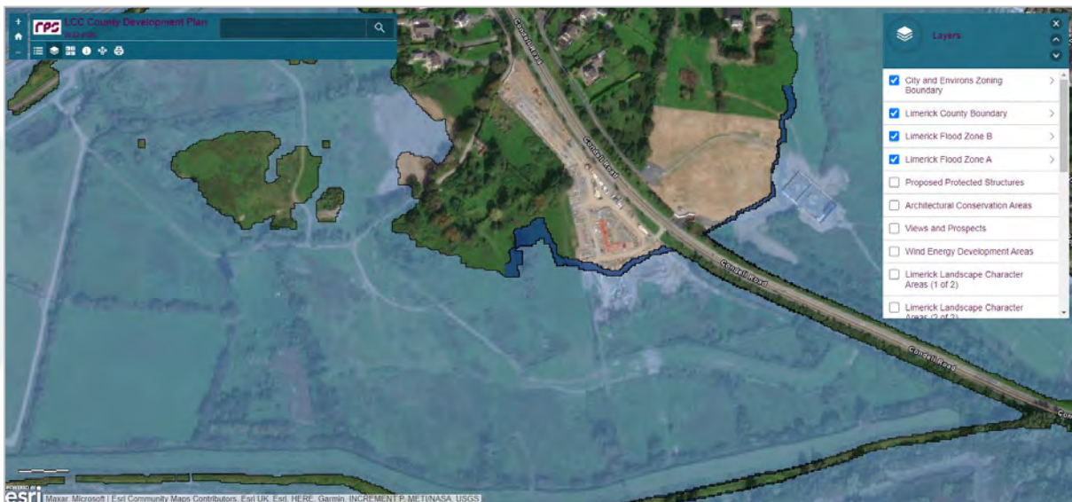
Figure 4: Flood Zones A (light blue colour) and B (dark blue colour) overlaid on aerial map. Source: LCCC Virtual Room - Interactive Map
