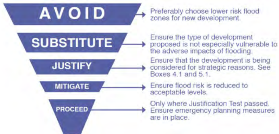
Figure 2-2: Sequential Approach Principles in Flood Risk Management
