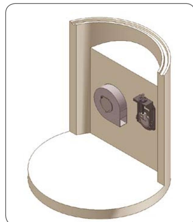
Figure 13 - 3D Section Showing Hydro-Brake® Chamber with Adjacent Penstock
