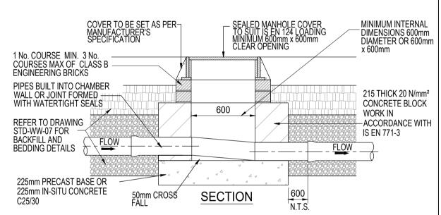
INSPECTION CHAMBER (BLOCK WORK CONSTRUCTION)
