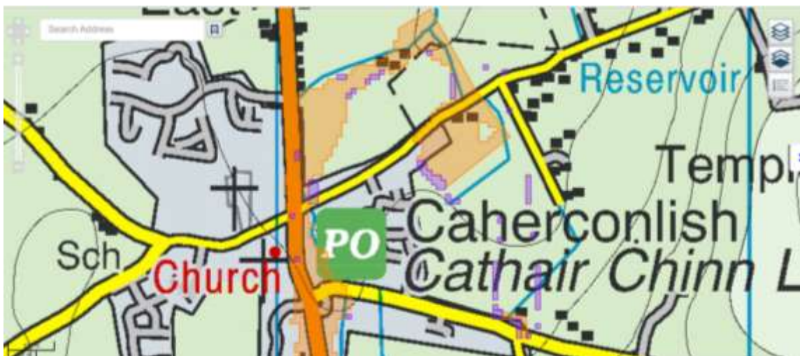
Figure 5: JBA flood mapping indicating Flood Zone A (Orange) and Flood Zone B (purple)
