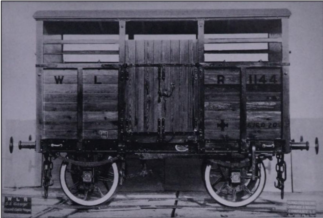
Figure 15. Covered cattle wagon of the Waterford and Limerick Railway, 1895.
