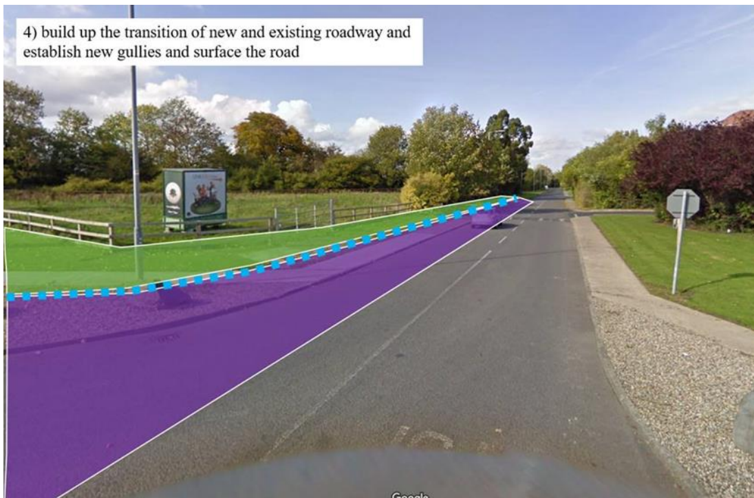
Figure 12: Construction Phase 4 © Google 2020
